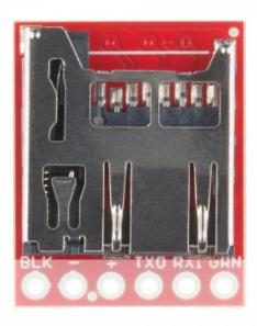
microSD Slot on the bottom of the OpenLog.
