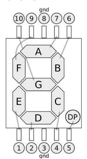
0-9 ten digits correspond with each segment are as follows (the following table applies common cathode seven segment display device, if you are using a common anode, the table should be replaced every 1 0 0 should all replaced by 1):
