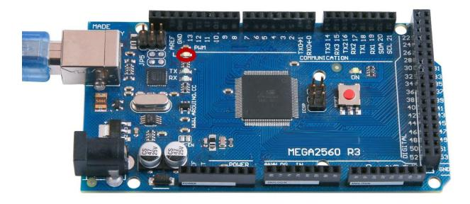
You may find that your MEGA2560 R3 board's 'L' LED already blinks when you connect it to a USB plug. This is because the boards are generally shipped with the 'Blink' sketch pre-installed.
