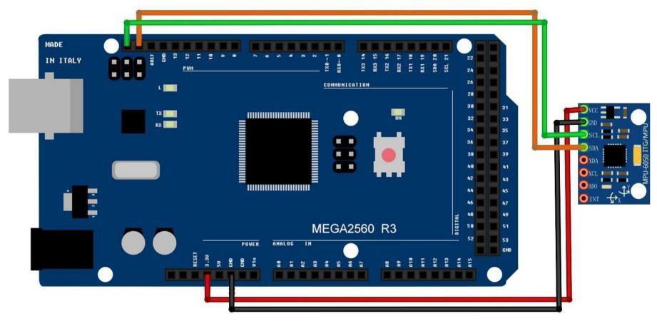
Next, we need to set up the I2C lines. For this connect the pin labelled as SDA on the GY-521 to the Arduino's analog pin 4 (SDA). And the pin labelled as SCL on the GY-521 to the Arduino's analog pin 5 (SCL). And that's it, you have finished wiring up the Arduino GY-521.
