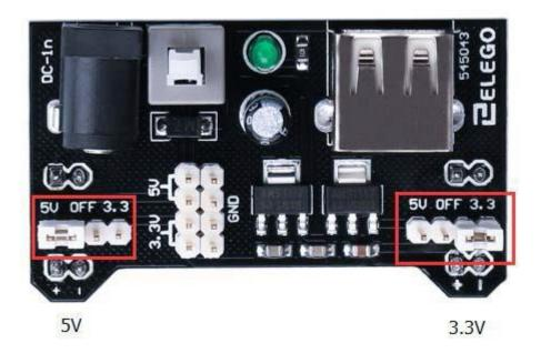
The left and right voltage output can be configured independently. To select the output voltage, move jumper to the corresponding pins. Note: power indicator LED and the breadboard power rails will not power on if both jumpers are in the "OFF" position.
