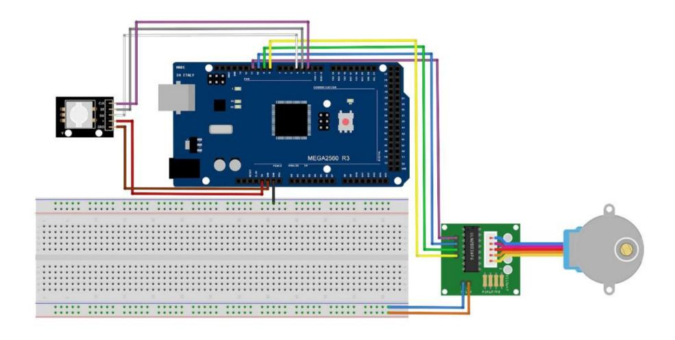
We are using 4 pins to control the Stepper and 3 pins for the rotary encoder module. Pins 8-11 are controlling the Stepper motor and pins 2-4 are receiving information from the rotary encoder.
