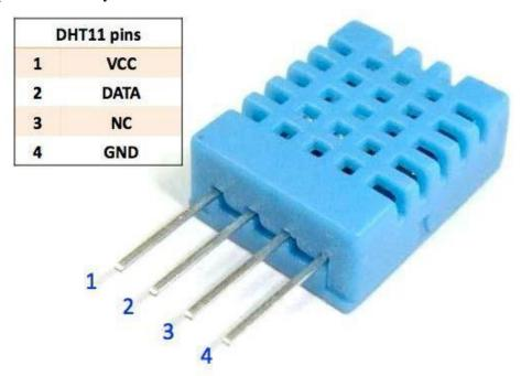
DHT11 digital temperature and humidity sensor is a composite Sensor which contains a calibrated digital signal output of the temperature and humidity. The dedicated digital modules collection technology and the temperature and humidity sensing technology are applied to ensure that the product has high reliability and
