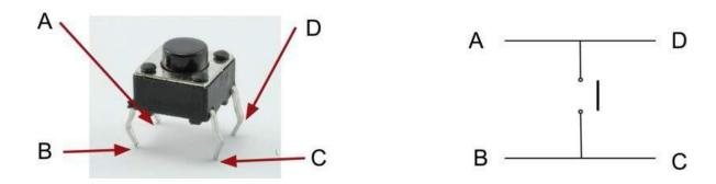
Actually, there are only really two electrical connections. Inside the switch package, pins B and C are connected together, as are A and D.
