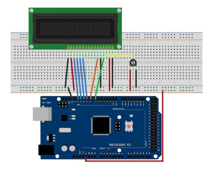
The LCD display needs six Arduino pins, all set to be digital outputs. It also needs 5V and GND connections.
