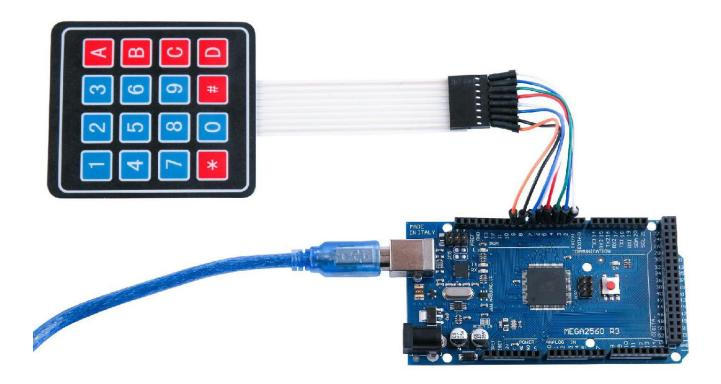
With this code, once we press a key on the keypad, it should show up on the serial monitor of the Arduino software once the code is compiled and uploaded to the MEGA2560 R3 board.
