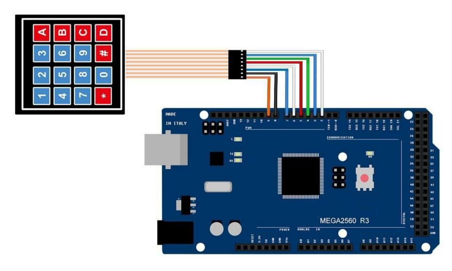
When connecting the pins to the MEGA2560 R3 board, we connect them to the digital output pins, D9-D2. We connect the first pin of the keypad to D9, the second pin to D8, the third pin to D7, the fourth pin to D6, the fifth pin to D5, the sixth pin to D4, the seventh pin to D3, and the eighth pin to D2.
