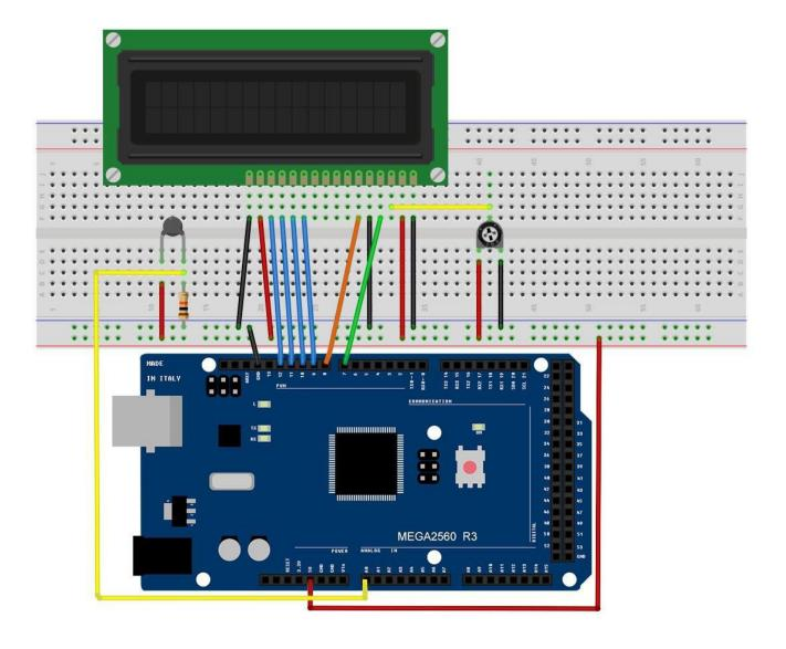
The breadboard layout is based on the layout from Lesson 22, so it will simplify things if you still have this on the breadboard.
