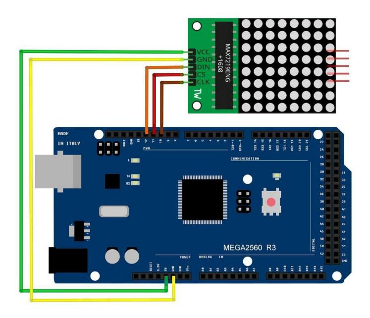
VCC and Ground are connected to the Arduino.
