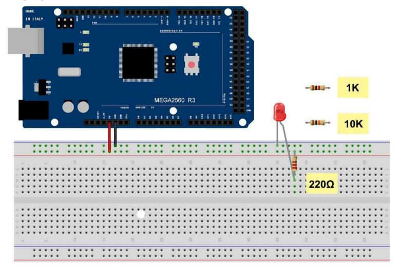
The MEGA2560 is a convenient source of 5 volts, which we will use to provide power to the LED and the resistor. You do not need to do anything with your MEGA2560, except to plug it into a USB cable.
