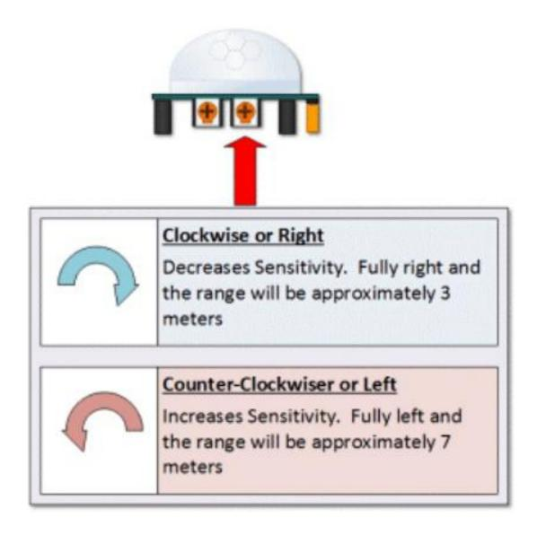
HC SR501 Sensitivity Adjust Time Delay Adjustment
