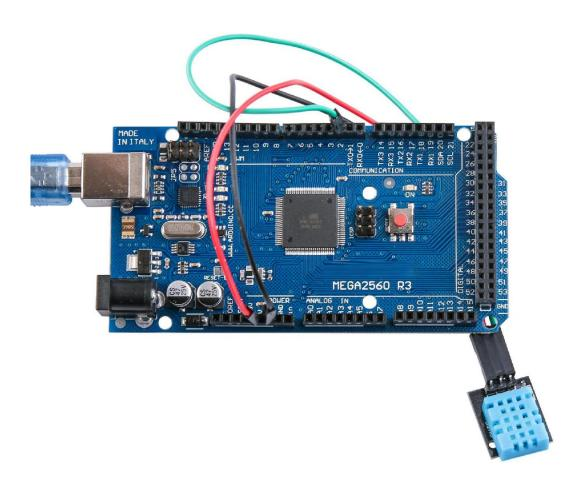
Upload the program then open the monitor, we can see the data as below: (It shows the temperature of the environment, we can see it is 22 degree)
