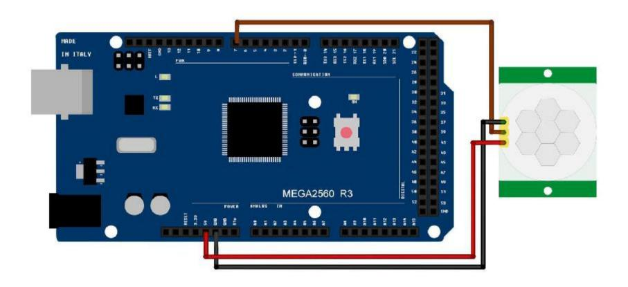
Connecting PIR sensors to a microcontroller is really simple. The PIR acts as a digital output so all you need to do is listen for the pin to flip high (detected) or low (not detected).
