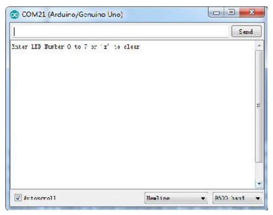
This window is called the Serial Monitor and it is part of the Arduino IDE software. Its job is to allow you to both send messages from your computer to an MEGA2560 board (over USB) and also to receive messages from the MEGA2560.
