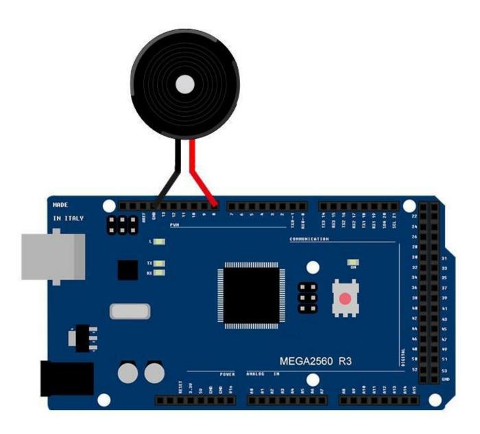
Wiring the buzzer connected to the MEGA2560 R3 board, the red (positive) to the pin8, black wire (negative) to the GND.
