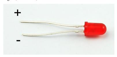
If you do not use a resistor with an LED, then it may well be destroyed almost immediately, as too much current will flow through, heating it and destroying the 'junction' where the light is produced.
