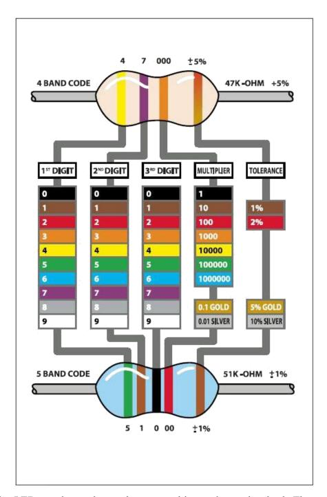
Unlike LEDs, resistors do not have a positive and negative lead. They can be connected either way around.
